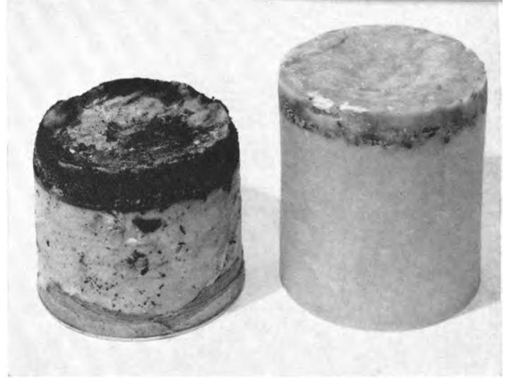
Solid fuel candle-type orchard heaters with cardboard containers removed. Candle on left burned for 12 hours.
