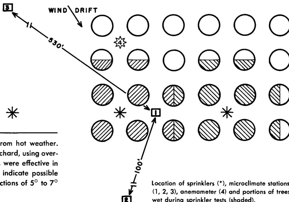
Location of sprinklers (\*), microclimate stations (1, 2, 3), anemometer (4) and portions of trees wet during sprinkler tests (shaded).
