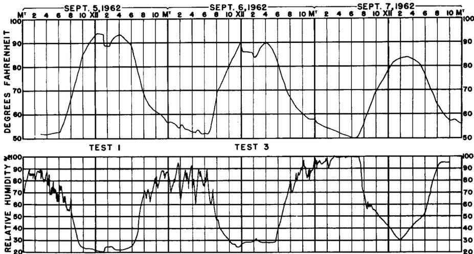
Hygrothermograph record showing air temperature (upper curve) and relative humidity (lower curve) changes in degrees Fahrenheit and per cent respectively for tests 1 and 3.
