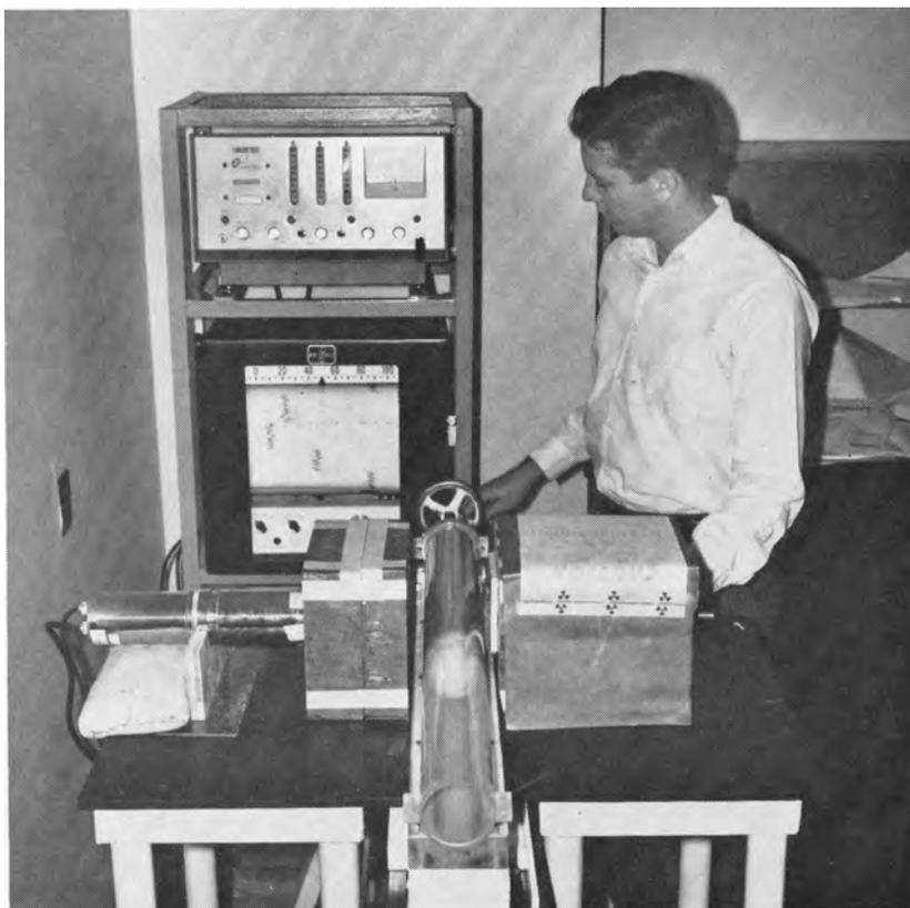
**T**he ability of soil to transmit water affects the rate, frequency and method of irrigation—and can often limit cropping possibilities in non-irrigated areas. Knowledge can be obtained on water movement through soil by measuring changes occurring after different periods of time. The gamma ray apparatus measures soil moisture on the basis that fewer gamma rays will pass through a wet soil than a dry soil.
