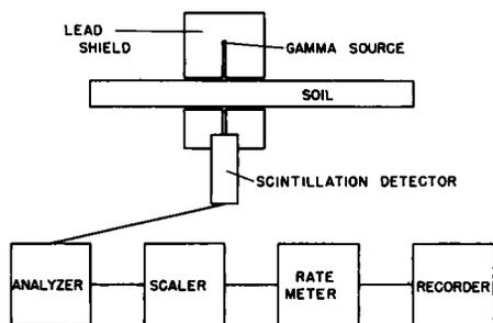
In addition to using the gamma ray device to understand how water moves through soil, it may be used directly for other problems in agriculture. Soil moisture extraction patterns by plant roots growing in greenhouse pots may be measured without plant disturbance. Soil compaction experiments may be carried out with great precision owing to the ability of the gamma device to measure bulk densities with extreme accuracy.
