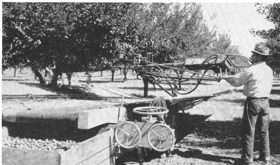
Inertia shaker mounted on self-propelled catching frame.
