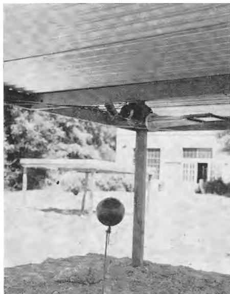
View under a test frame showing black globe thermometer used to measure radiant heat load and hemispherical radiometer to measure radiation received by underside of test material.
