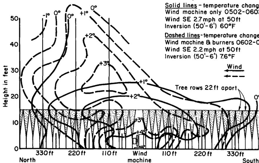
Vertical cross-section showing the temperature changes (°F) on March 25, 1959. Note the schematically presented trees and the solid heavy vertical lines which indicate the masts for the temperature sensing instruments.
