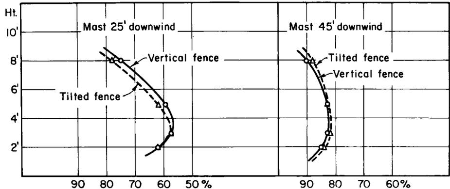
Velocity in percent of outside wind velocity along two masts on lee side of a 6' snow fence, 25% pervious, average of 5 tests in April, 1959.
