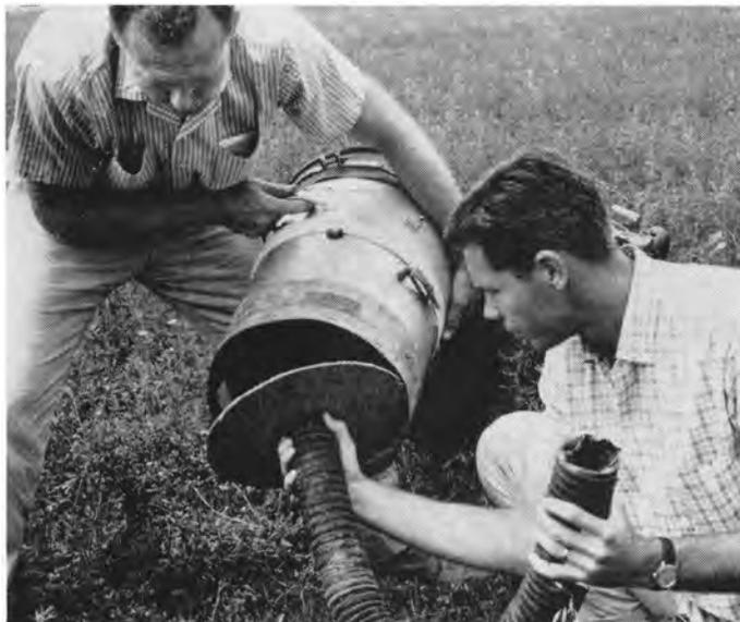
**Placement of adapter hose for complete sampling.**
