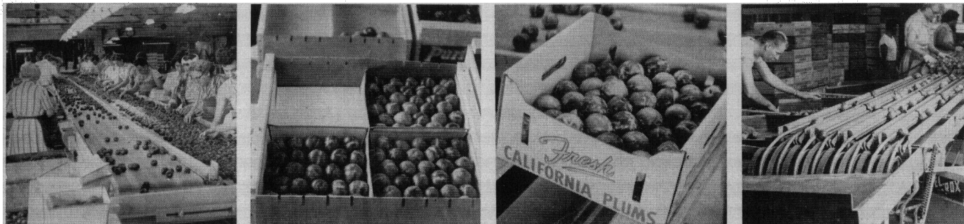
Left—conventional place-pack from moving belt; fruit sized visually by packer and placed individually in container. Left center—standard four-basket crate, 28 pounds net weight. Right center—test carton, 25 pounds net weight. Right—equipment for rope-sizing fruit into bins for place-packing, modified to permit bulk-fill of container.
