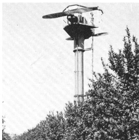
Typical dual-engine wind machine in a citrus orchard.
