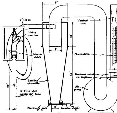
Schematic drawing of the sampling device.
