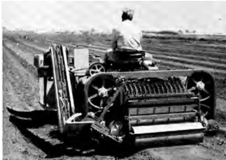
Cutting blade, conveyor, and roller of the second model asparagus harvester.
