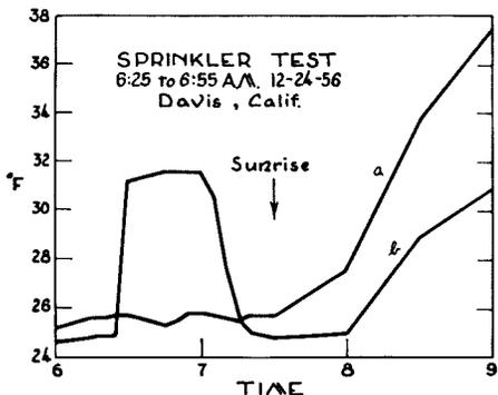
Temperature rise during sprinkling—curve a. As operation was stopped before sunrise the sprinkled bulb cooled to previous temperature and stayed colder than the outside control bulb—curve b—until the ice crust had melted and the water had evaporated.
