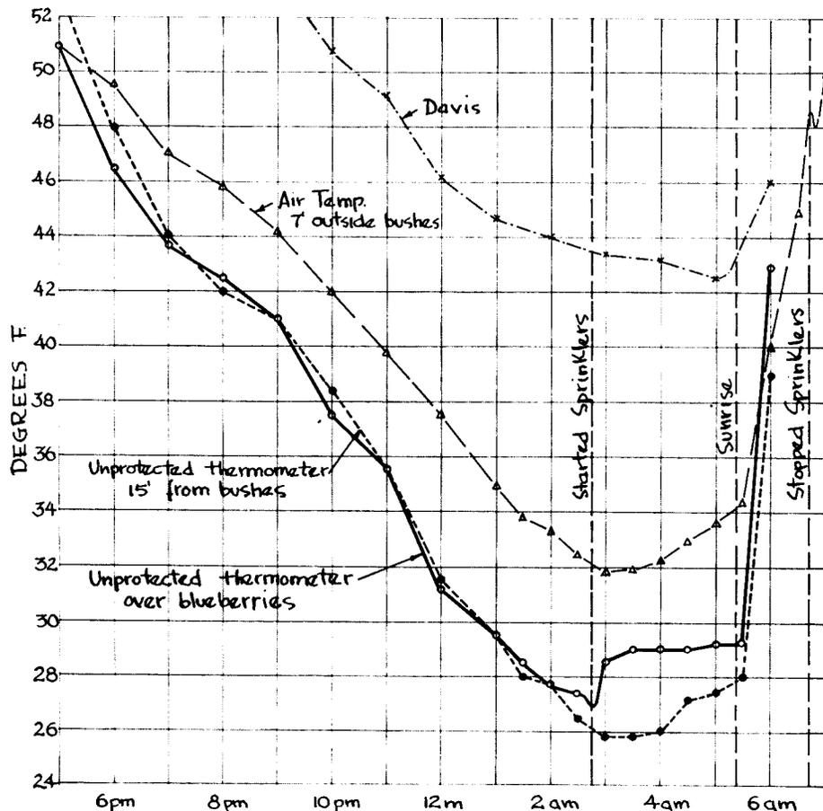
Wind trouble at stations c and d diminished water supply making frost protection insufficient. Only station b got full amount—0.08" per hour rain. Curve a represents outside control bulb. After sprinkler was turned off at sunrise, strong evaporation cooling due to dry wind caused a temperature drop to 3°F lower than before operation started.
