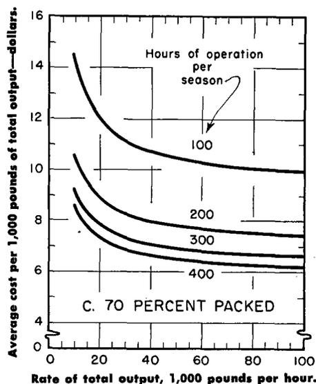
The effect of capacity rate of output—size of plant—and hours of operation per season on average costs per 1,000 pounds of total fruit run. Packed fruit, 70% of total run; 1954 price level. Package materials costs are excluded but are estimated to be about 60¢ per standard box—48 pounds net weight. Inclusion of package materials costs would increase the level of cost in the diagram by about \$8.75 per 1,000 pounds.
