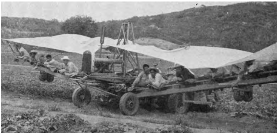
The wings of the machine can be raised at the end of the row in preparation for turning.
