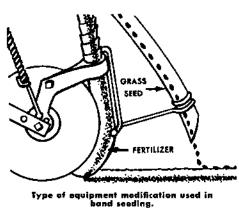
ment and a fertilizer box. Rubber hoses attached to the grass seeder box made it possible to direct the seed into the furrow directly over the band of fertilizer placed 4" into the ground. As the furrow made by the disks closed, the seed was dropped on top of the ground and covered with a drag chain.
