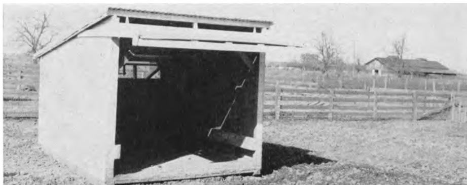
Three-sided shade 6' high for observation of effect of walls on radiation heat load.
