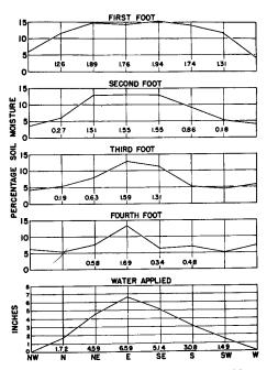
Distribution of soil moisture from sprinklers in a pear orchard where low branches interfered with uniform delivery.
