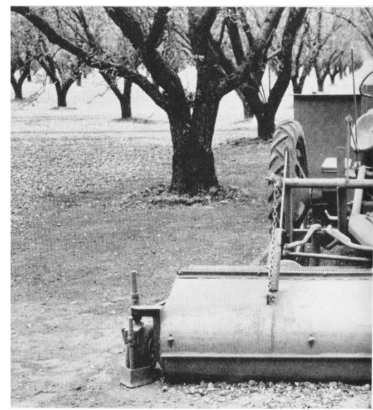
Newly designed prune catcher is pushed by tractor onto conveyor belts to be carried
