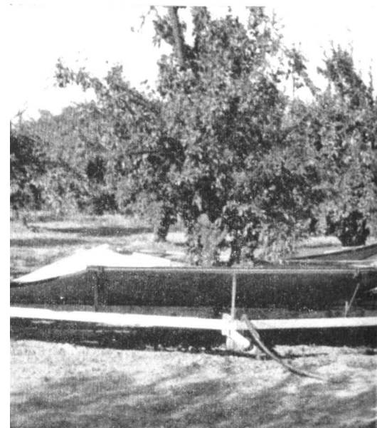
Newly designed prune catcher is pushed by tractor onto conveyor belts to be carried
