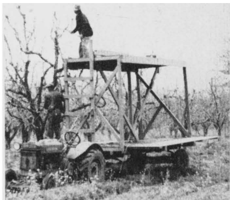
Two-stage pruning platform for pears with slipboards on upper deck. Compressor is mounted on tractor.
