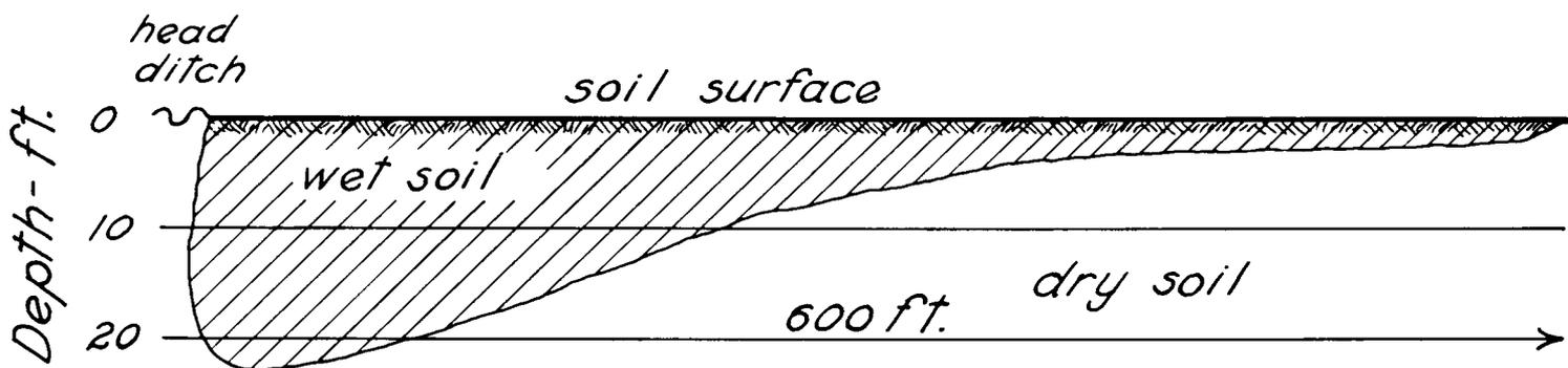
Deep percolation, or waste of water near the head ditch. A small flow of water requires a long time to reach the end of the run.
