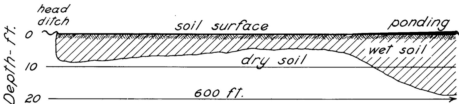
Deep percolation from ponding at the end of the run. Too large a flow was used with resultant ponding and wasting of water.
