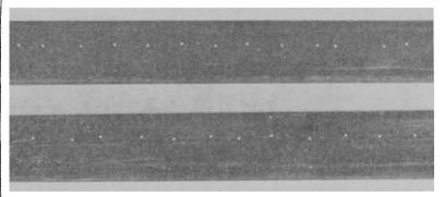
In the above illustration the white spots are seeds on boards coated with heavy grease to hold the seeds in place. In the laboratory tests these greased boards were used to catch the seed as it was dropped by the planter and to hold them where they fell so the accuracy of the mechanism could be studied.
