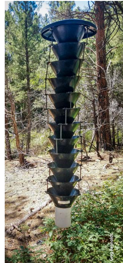
A funnel trap baited with the pheromone pityol was used to trap twig beetles. The pitch canker pathogen was recovered from insects on eight of 14 sampling dates, at levels that ranged from 0.1% to 4%.
