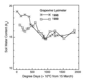
Fig. 2. Mean soil water content (expressed as percent by volume:  $\theta_v$ ) measured in the weighing lysimeter during the 1998 and 1999-growing seasons. An individual data point is the average of two access tubes measured at six depths (from 0.23 to 1.65 m below the soil surface).
