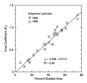
Fig. 10. The crop coefficient ( $K_c$ ) of Thompson Seedless grapevines growing in the weighing lysimeter as a function of the percent shaded area measured beneath the two vines. The  $K_c$  was calculated by dividing grapevine ET<sub>c</sub> (mm per day, from Fig. 7) by reference ET (ET<sub>o</sub>) on the day the shaded area was measured.
