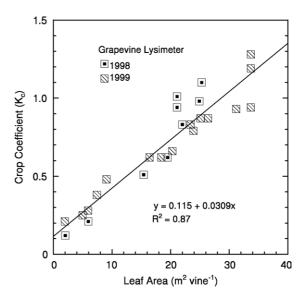
Fig. 8. The relationship between the calculated crop coefficient ( $K_c$ ) and the estimated leaf area per vine of Thompson Seedless grapevines growing in the lysimeter during 1998 and 1999. The  $K_c$  data was calculated by dividing grapevine ET<sub>c</sub> (mm per day) by reference ET (ET<sub>o</sub>) on the day the leaf area was determined.
