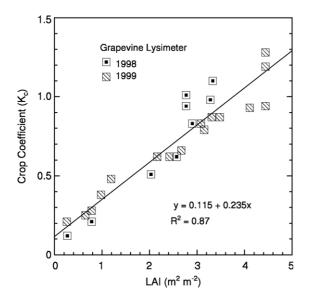
Fig. 9. The relationship between the calculated crop coefficient ( $K_c$ ) and the estimated leaf area index (LAI) of Thompson Seedless grapevines growing in the lysimeter determined during 1998 and 1999. The LAI was determined by dividing the leaf area by 7.55 m<sup>2</sup>, the area allotted per vine in the vineyard surrounding the lysimeter. Other information is as given in Fig. 7.
