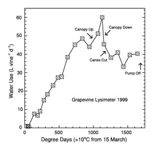
Fig. 3. Daily water use of Thompson Seedless grapevines measured from March 15 until the irrigation pump to the lysimeter was turned off on September 2 (1746 DDs after March 15) in 1999. Each data point is the average daily value for a 7-day period. The arrows represent the approximate days when the north and south portions of the canopy were raised or lowered and when the apical portions of the shoots were hedged (canes cut), approximately 0.45 m above the soil surface.
